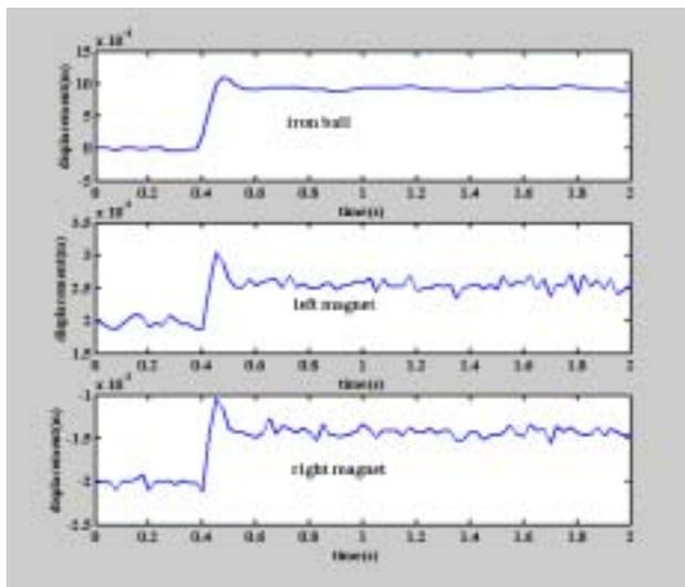
Fig.8. Step response of experimental examination of  $K_1$
