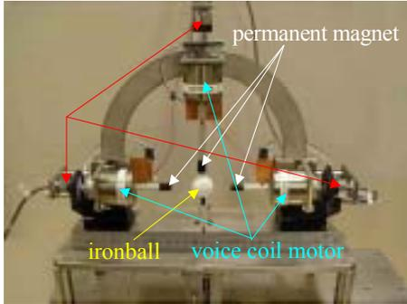
Fig.2. The prototype of system
