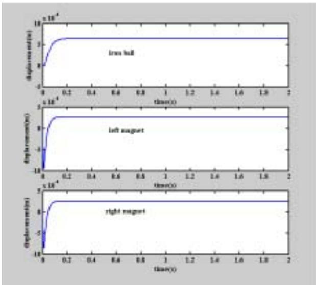
Fig.6. Step response of numerical simulation of  $K_1$
