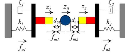
Fig.4 Horizontal motion model of system
