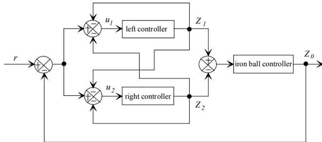
Fig.5 The control system block diagram
