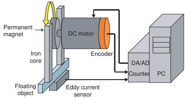
Fig. 3. Illustration of control system for a prototype suspension system.
