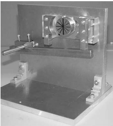
Fig. 2. Photograph of a prototype suspension system.
