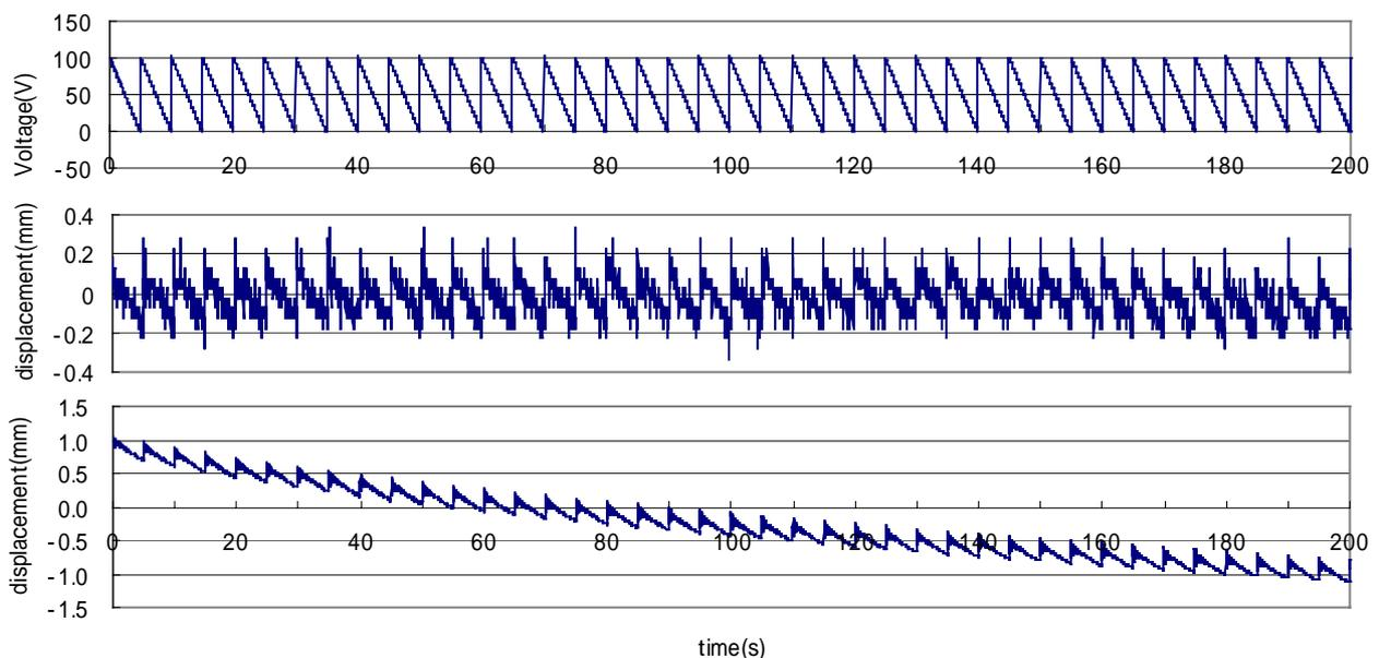
Fig.9. Supplied voltage displacement of superconductor, displacement of permanent magnet
