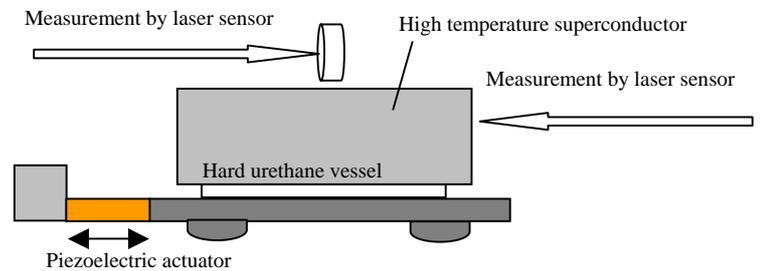
Fig.6. Impact driving experimental system
