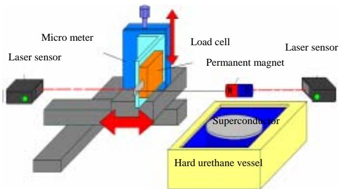
Fig.3. Pinning force measurement system
