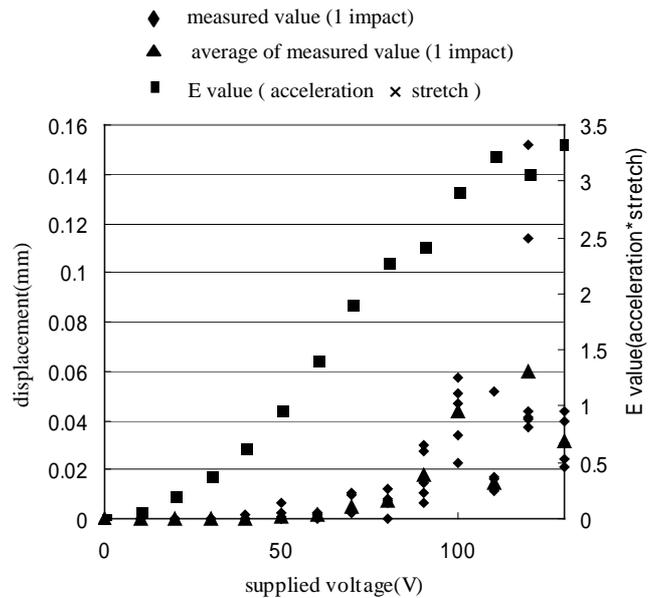
Fig.8. Relation with supplied voltage, permanent magnet's displacement and E value
