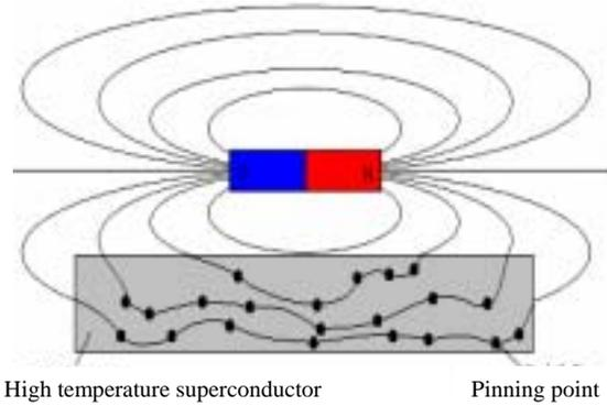
Fig.1. Pinning point and normal conduct positioning
