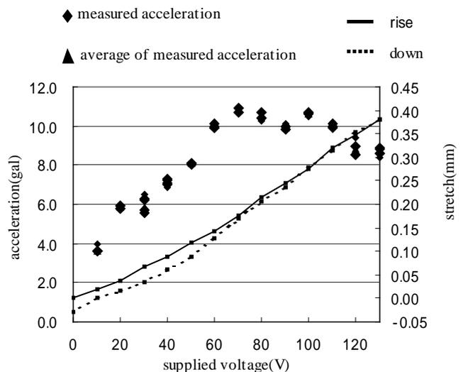
Fig.7. Performance of piezoelectric actuator
