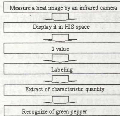
Fig.2 Algorithm of the recognition
