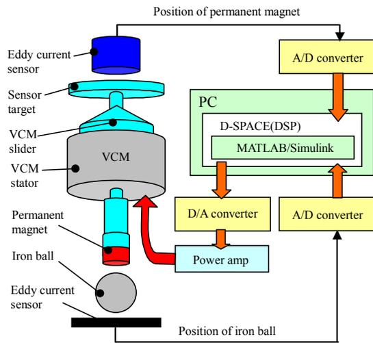
Figure 3: Configuration of Magnetic Suspension System
