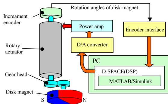
Figure 4: Configuration of One Spinning System
