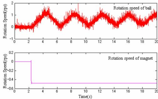
Figure 8: Step response of iron ball using two disk magnets
