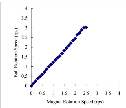
Figure 14: Relationship between magnet velocity and iron ball velocity (two magnets)
