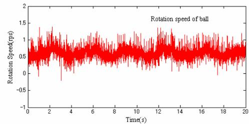
Figure 11: Steady state velocity of iron ball using two disk magnets
