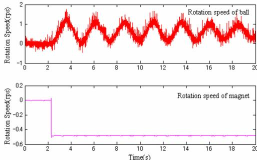
Figure 9: Step response of iron ball using four disk magnets
