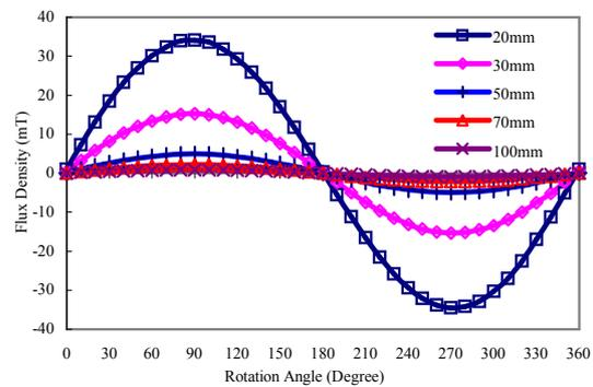
Fig. 6 Magnetic Flux Density Characteristic of Disk Magnet
