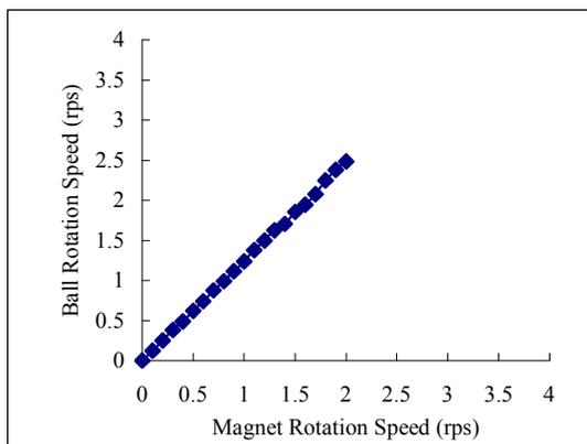
Figure 15: Relationship between magnet velocity and iron ball velocity (four magnet)
