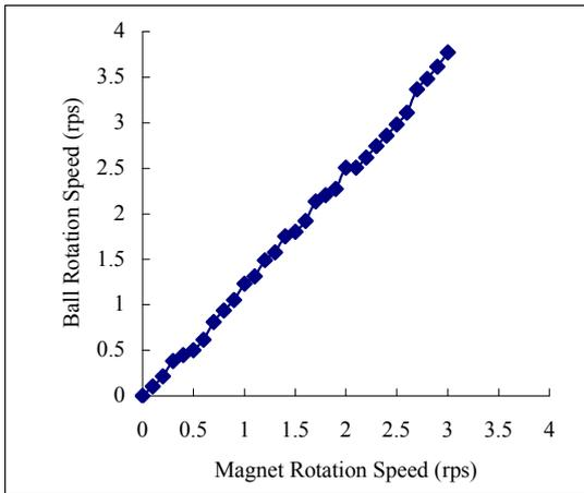
Figure 13: Relationship between magnet velocity and iron ball velocity (one magnet)
