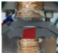
Fig.5 Illustration of rotor width of teeth  $30^\circ$
