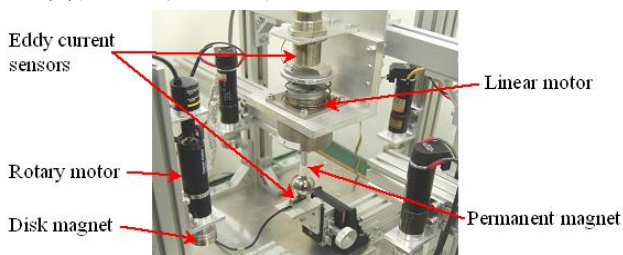
Fig.1 Rotation Driving Type Mechanism
